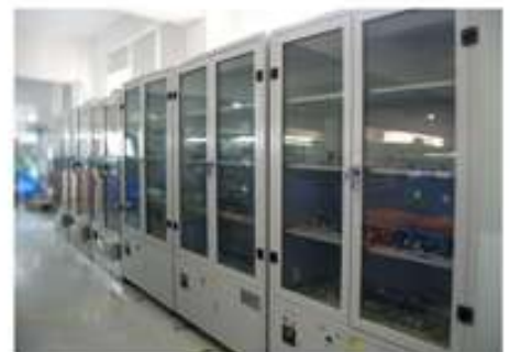
PCB burn-in test
